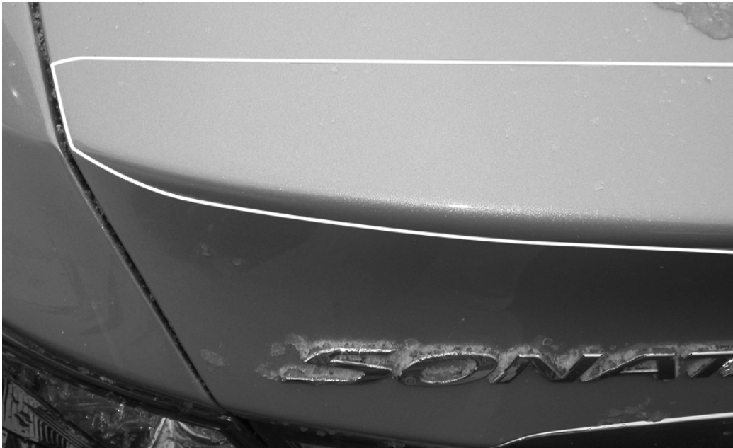
Outline marks on deck lid made in Step #2. Repeat on passenger side.
