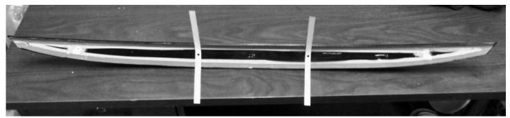
When Sportwing® is centered on outline marks made in Step #2, and making sure that the two (2) paper hole locators did not move, tape all two (2) paper hole locators to the deck lid using masking tape. Next, carefully lift the Sportwing off the deck lid, leaving the hole locators taped to the deck lid.
