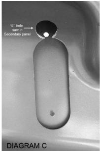
Open deck lid and using a <sup>3</sup>/<sub>4</sub>" hole saw, open 5/32" pilot hole that you made in secondary panel to <sup>3</sup>/<sub>4</sub>" Black <sup>3</sup>/<sub>4</sub>" hole caps have been provided for these holes upon finishing.
