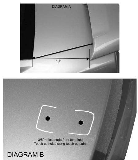
Outline both mounting feet using grease pencil. Using template, provided, drill 5/32" or similar pilot hole on designated spots on template (**NOTE**: when drilling rear most hole on template you will need to continue drilling through secondary panel of inner deck lid). Next, using a uni-bit (**NOTE**: we suggest using a uni-bit for a cleaner cut) open the 5/32" pilot holes on top panel to 3/8", as shown above).
