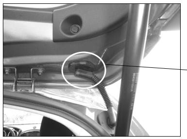
Remove plug for access to the top panel of the hatch on passenger and driver's side. Replace upon finishing installation.
