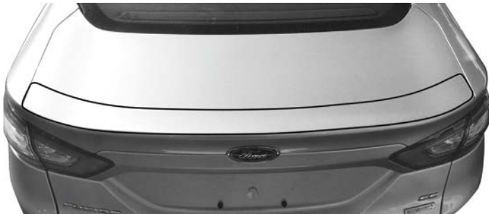
DIAGRAM B: Outline spoiler with a grease pencil
