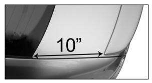
2. Place the Sportwing® on the marks made in Step #1. **See diagram below**. As you face the rear of the car, the front tips of the Sportwing® will rest on these marks. Center the Sportwing® exactly from left to right. Using a yellow grease pencil, completely outline the Sportwing®. Remove the Sportwing® from the trunk.
