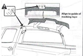
**STEP 5:** Using the marked position on the masking tape from step 2 as a guide, carefully align the cab spoiler to the roof.
