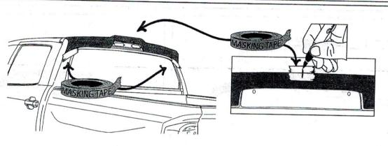
STEP 3: Peel back approximately 50mm (2" in) of tape liner from each of the tape sections and fold liner at 45 degrees to the outside of cab spoiler. Using a blade carefully cut the tape liner in the center of part and peel back at 45 degrees, tape all peeled back sections of tape liner to the outside of cab spoiler using masking tape.
