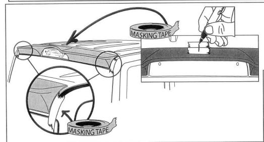
**STEP 3:** Place masking tape on roof aligning the edge of the masking tape to each end on the cab spoiler. Place masking tape centrally on the roof sheet metal and cab spoiler, mark line with a non-permanent pen to assist in positioning.
