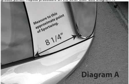
2. <u>Leaving the paper on the bottom of the mounting feet, place the Sportwing® on the marks made in step #1 so that as you face the rear of the car, the front edge as shown of the Sportwing® rests on the mark. Center the Sportwing® from left to right. Using a yellow grease pencil, outline both mounting feet. Set the Sportwing® aside.</u>
