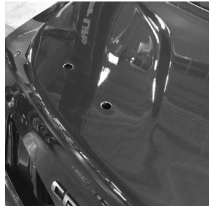
2 of 4 Drilled Spoiler Holes
