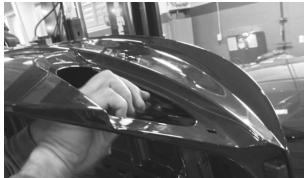
Screwing Spoiler into Deck Lid >
