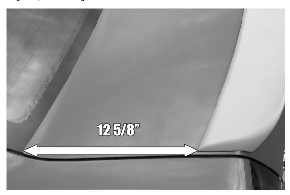
4. Place Sportwing® on trunk and align tips of spoiler with the marks you just made in the previous step, center spoiler, and outline the spoiler using your grease pencil for placement later in installation.
