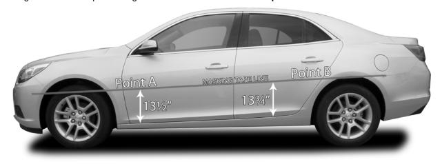
Measure up from bottoms of doors; measure before door curves upward for rear door.
