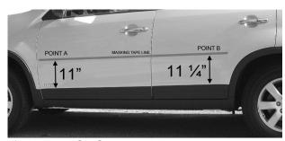
If model DOES have cladding, measure up from top of cladding.
