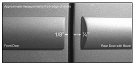
APPLY THE MOLDING the top of the molding should follow along the bottom of your masking tape line, which is your guide; peel off the rest of the red liner as you go.
