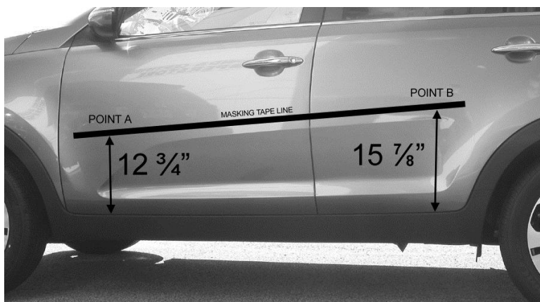
Measure up from bottom of doors
