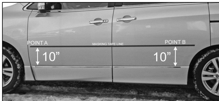
Measure up from top of cladding
