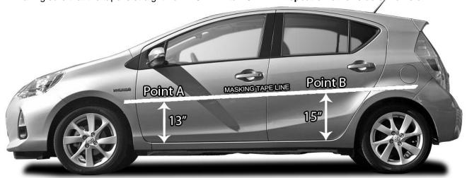
Measure up from bottom of door. For rear measurement, measure before door curves upward.
