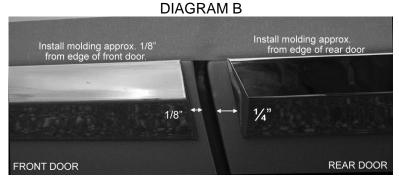
4. <u>AFTER THE MOLDING</u> has been installed, use a soft cloth and apply pressure along the entire length of the molding to insure proper adhesion.
