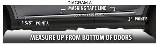
Measure up from the bottom of the doors to the bottom edge of the masking tape.
