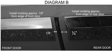
4. <u>AFTER THE MOLDING</u> has been installed, use a soft cloth and apply pressure along the entire length of the molding to insure proper adhesion.
