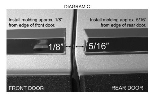
4. <u>AFTER THE MOLDING</u> has been installed, use a soft cloth and apply pressure along the entire length of the molding to insure proper adhesion.
