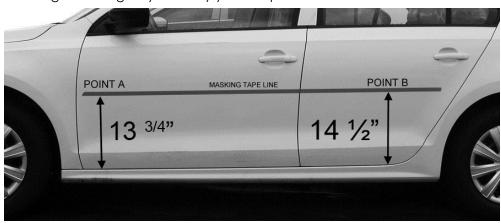
\*Measure up from bottom of doors. Top of molding should meet bottom of tape line.\*
