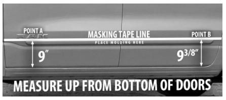
(The Crew Cab is shown in image to the left, the Quad Cab is not pictured. However, the Crew Cab and the Quad Cab use the same "measure-ups". Please note that the Moldings themselves are different lengths but use the same "measure ups.")
