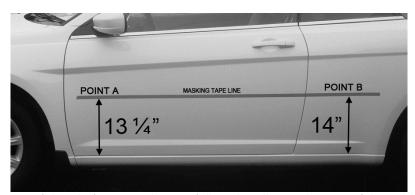
Measure up from bottom of door in front, continue to follow door line to the rear of the vehicle and measure up.
