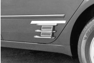
Use masking tape to guide the placement and installation of each Sportstyle™ Vent.
