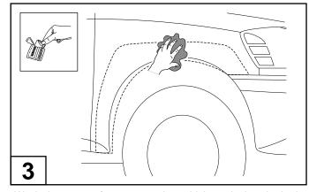
Wash the areas of contact on the vehicle and wipe dry both the vehicle and the Fender Flares with a clean cloth. Ensure inside of Fender Flares where extrusion is attached is clean, use alcohol wipe supplied to clean surface.
