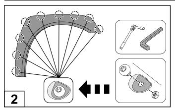
Attach 9 bolts to each Fender Flare using a 3/16" Allen key and a 1/2" wrench/socket. (wrench/socket and Allen key not supplied)
