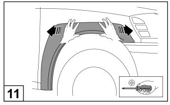
If necessary, make minor adjustments to the flare's position to achieve the best fit for your vehicle. Once satisfied, tighten all screws currently installed.
