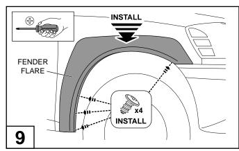
Place flare on vehicle and attach the four (4) previously removed screws as shown. Do not fully tighten at this stage.
