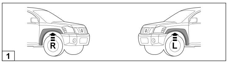
Ensure that both left and right hand Fender Flares suit the profile of the vehicle. Note the areas where the Fender Flares come in contact with the vehicle. **NOTE:** Before fitting Fender Flares remove any mouldings, strips or existing flares from the wheel arch. If there is a body side moulding, mark where the moulding is to be cut, alternatively the Fender Flares can be cut to go around the moulding. Be sure to allow enough room for the extrusion.
