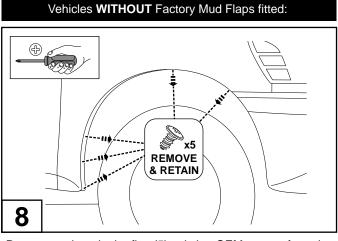
Remove and retain the five (5) existing OEM screws from the wheel arch.
