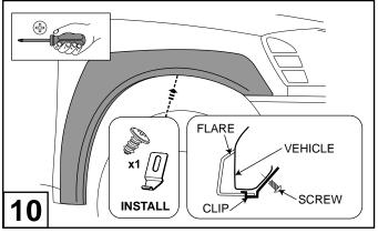
Locate the clip in the slot on the flare as shown. Secure to vehicle using the previously removed screw.
