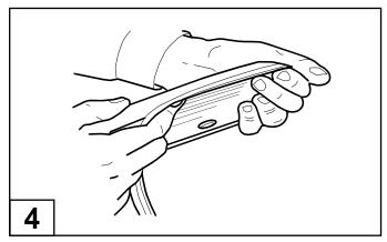
Remove approximately 2" (50mm) of the protective liner from the extrusion. Fit the extrusion to the Fender Flare along the edge that comes in contact with the vehicle's body panel. **NOTE: Do not use this extrusion for the rear flare**
