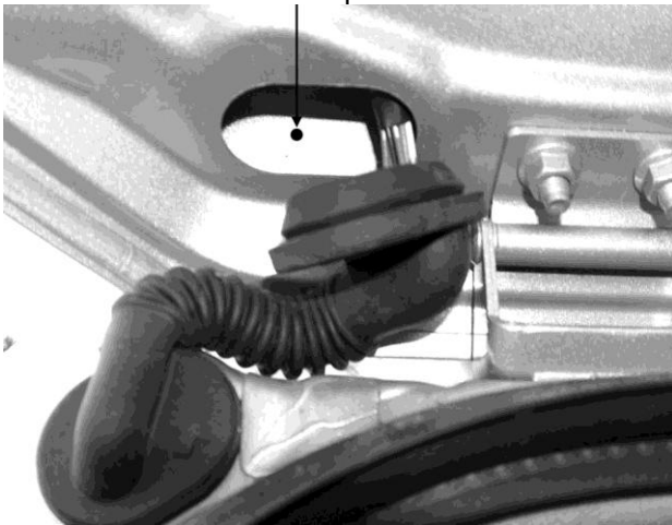
DIAGRAM D Drivers side 5/32" hole in top panel of hatch made from TEMPLATE in Step #3.
