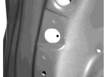
Close up of off center 5/32" hole.
