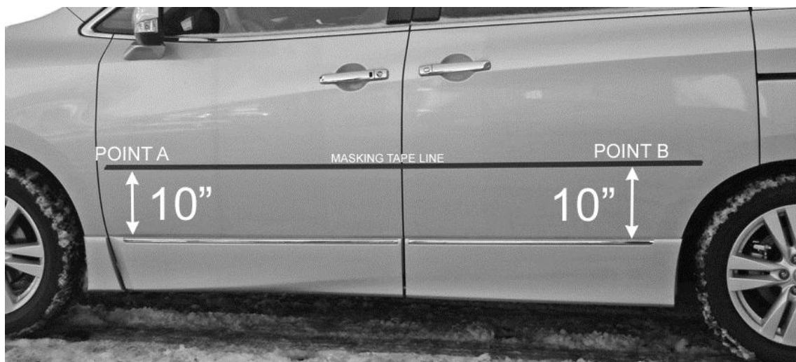
Measure up from top of cladding
