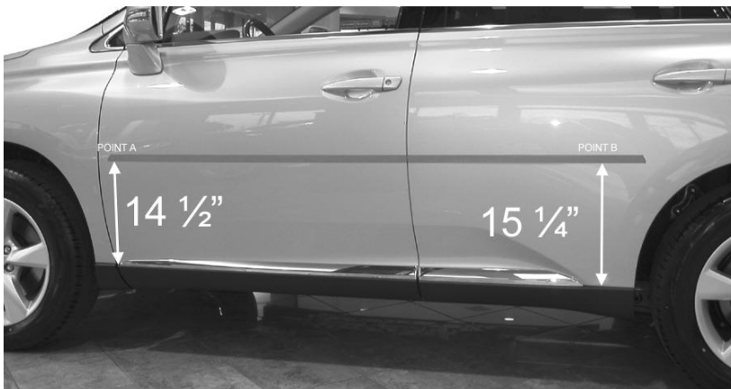
Measure up from top of black cladding
